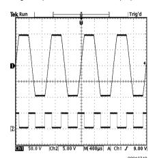
$+V_{CC}$  =  $-V_{EE}$  = 100V,  $V_{IN}$  =  $4V_{RMS}$ ,  $f_{IN}$  = 1kHz,  $R_{C}$  =  $1k\Omega$ Ch1: Output, Ch2: CLPFLAG Output
