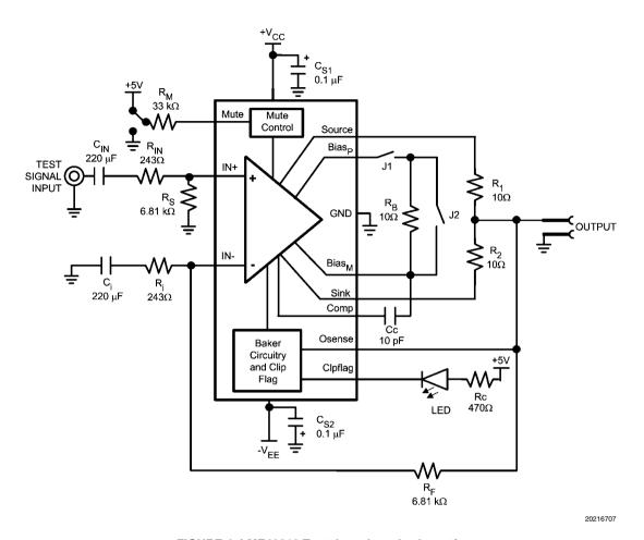
FIGURE 4. LME49810 Test demo board schematic
