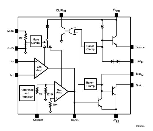
FIGURE 2. LME49810 Simplified Schematic
