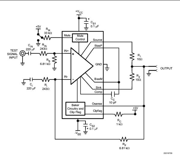
FIGURE 3. LME49810 Test Circuit Schematic (DC Coupled)
