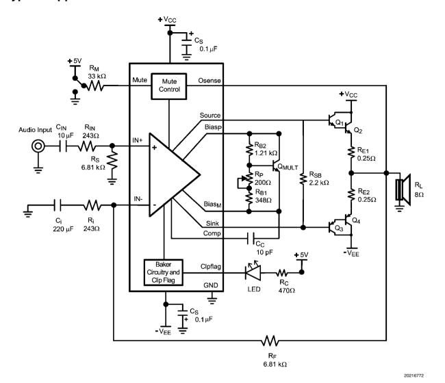
FIGURE 1. LME49810 Audio Amplifier Schematic
